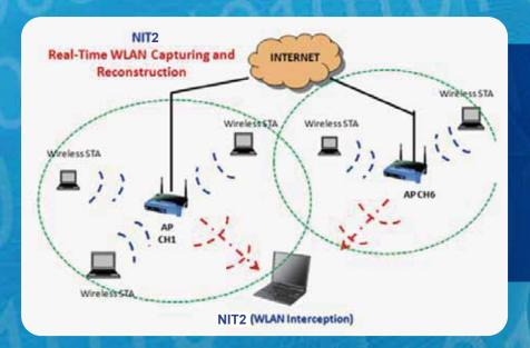
Single System with Multiple High Gain Antenna for Wi-Fi Traffic Monitoring by Different Channels
